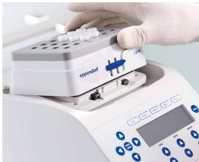
SmartBlock removal from Eppendorf ThermoMixer® C
